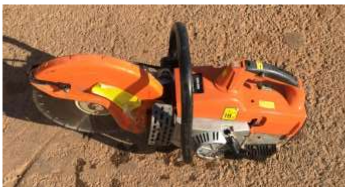
Concrete cut off saw
