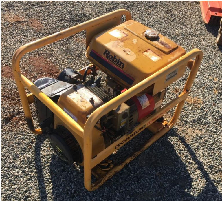
Robin 5KVA generator
