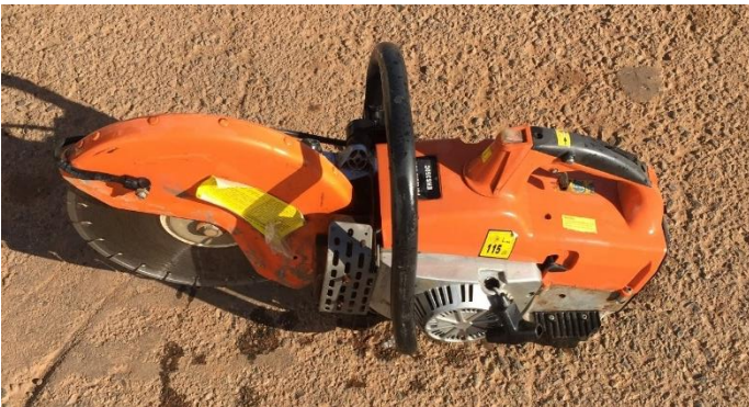
Concrete cut off saw
